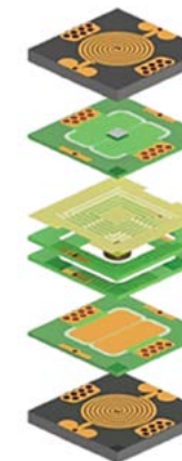
The process of heterogeneous integration involves the separate manufacturing of components, which are later assembled together.
