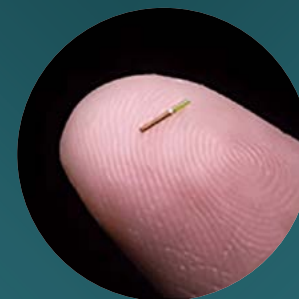
The eyelash-size, battery-free, biocompatible pressure sensor to measure pressure in the eye.
